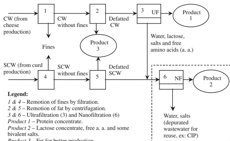
Fig. 1. Process for nutrients recovery and valorization of “Serpa” cheese by-products.
