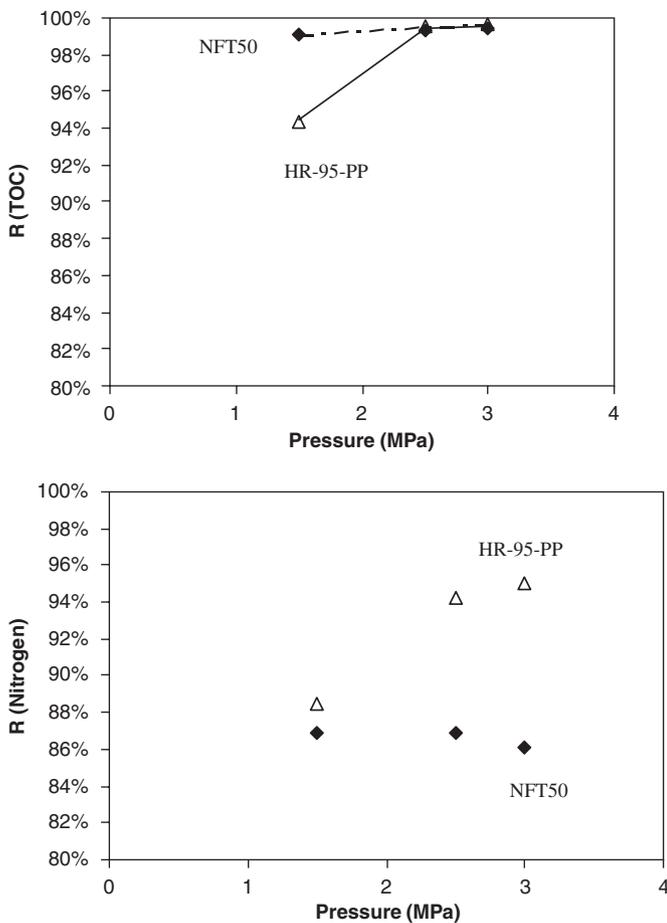
Fig. 3. Variation of the TOC rejection (a) and total nitrogen rejection (b) with the applied pressure—total recirculation mode.
