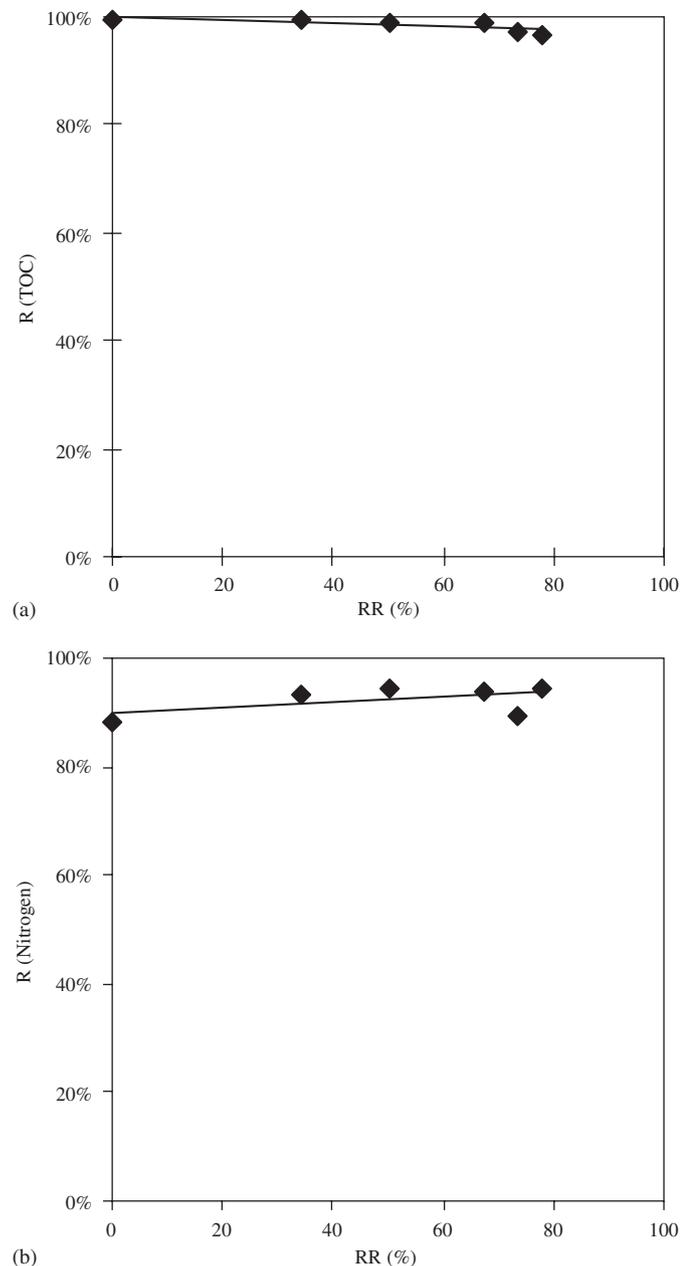
Fig. 5. Variation of the TOC rejection (a) and total nitrogen rejection (b) with the water recovery rate—concentration mode. Membrane: NFT50, pressure: 3.0 MPa.
