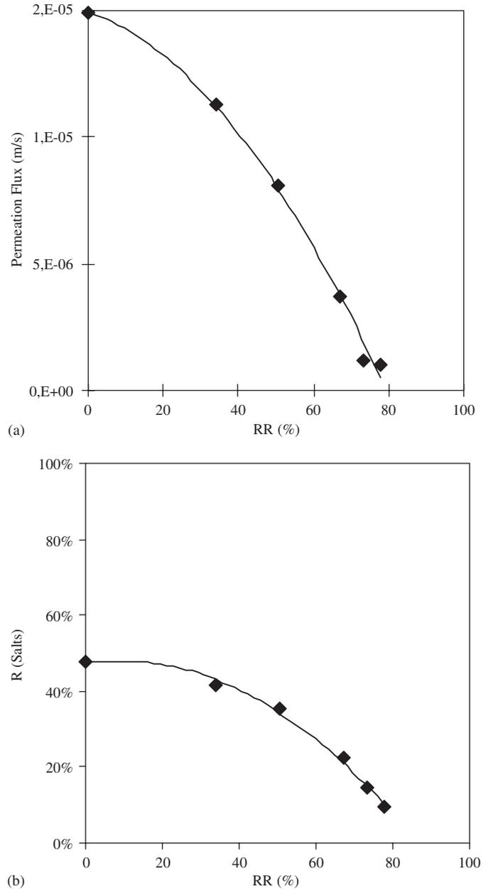
Fig. 4. Variation of the permeation fluxes (a) and salts rejections (b) with the water recovery rate—concentration mode. Membrane: NFT50, pressure: 3.0 MPa.
