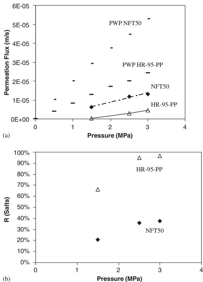
Fig. 2. Variation of the permeation fluxes (a) and salts rejections (b) with the applied pressure—total recirculation mode.
