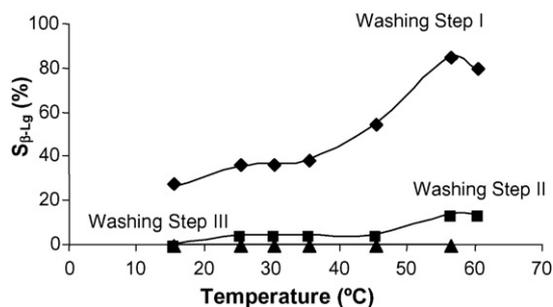
Fig. 3. Influence of temperature on the solubilization degree of  $\beta$ -Lg (S) after three successive washing steps performed with acidulated fresh water at a pH value of 4.0.
