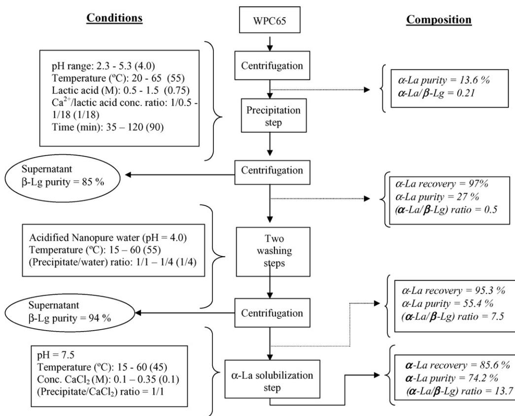
Fig. 1. Flowsheet of the proposed process to obtain a liquid stream enriched in  $\alpha$ -La. The values between brackets represent the optimum value of the corresponding variable.
