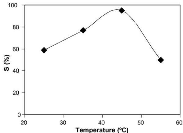
Fig. 5. Influence of temperature on the solubilization degree (S) of  $\alpha$ -La when the precipitate was washed with a solution of 0.1 M  $\text{CaCl}_2$  at a pH value of 7.5.
