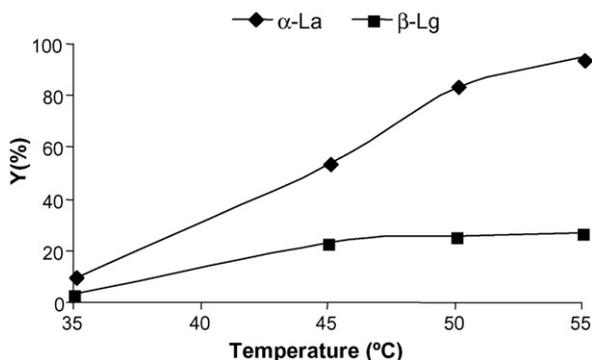
Fig. 2. Precipitation yield (Y%) of  $\alpha$ -La and  $\beta$ -Lg vs. temperature. Operating conditions: pH 4.0; lactic acid concentration = 0.75 M.
