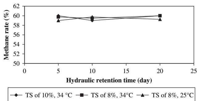
**Fig. 8 – Methane rates of biogas for the mixtures including 8% and 10% TS at different HRTs.**
