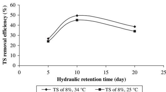
**Fig. 10** – TS removal efficiency for the mixture including 8% TS at different HRTs and temperatures.
