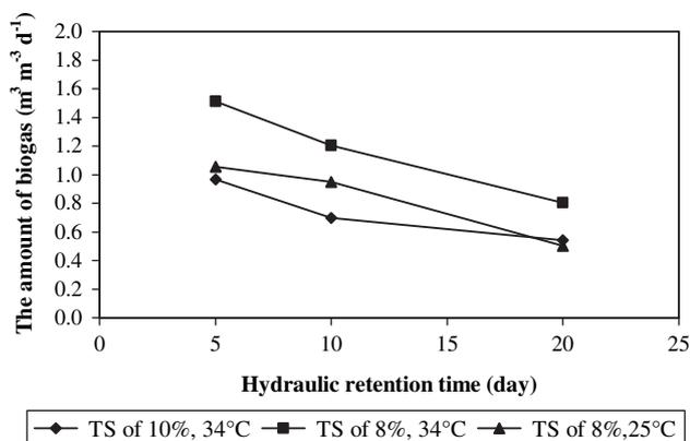
**Fig. 7 – Biogas production rates for the mixtures including 8% and 10% TS at different HRTs.**
