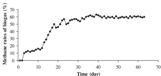
Fig. 4 – Daily methane rates of biogas at 34 °C and 8% TS.
