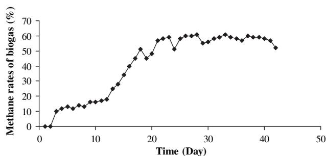
Fig. 6 – Daily methane rates of biogas at 25 °C and 8% TS.
