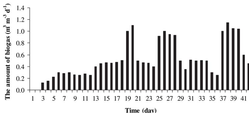
Fig. 5 – Daily biogas production rates at 25 °C and 8% TS.
