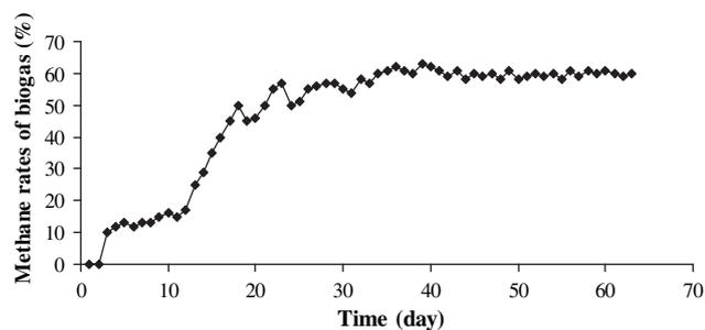
Fig. 2 – Daily methane rates of biogas at 34 °C and 10% TS.
