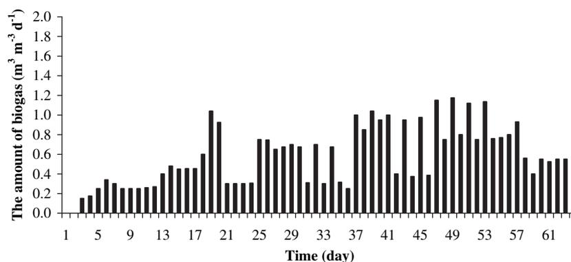
**Fig. 1 – Daily biogas production rates at 34°C and 10% TS.**
