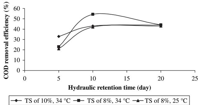
**Fig. 9** – COD removal efficiency for the mixtures including 8% and 10% TS at different HRTs.
