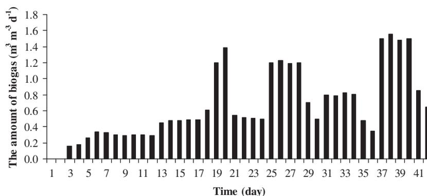
**Fig. 3 – Daily biogas production rates at 34 °C and 8% TS.**
