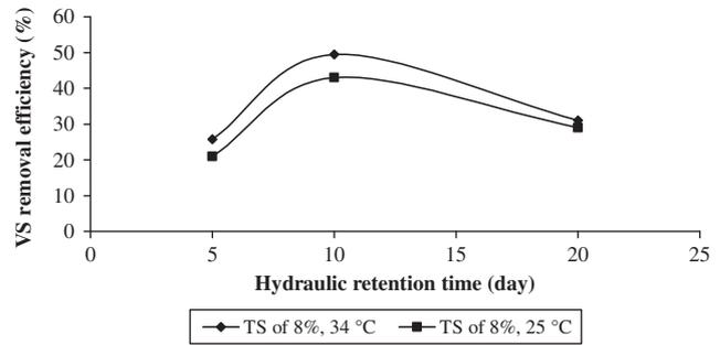
**Fig. 11** – VS removal efficiency for the mixture including 8% TS at different HRTs and temperatures.
