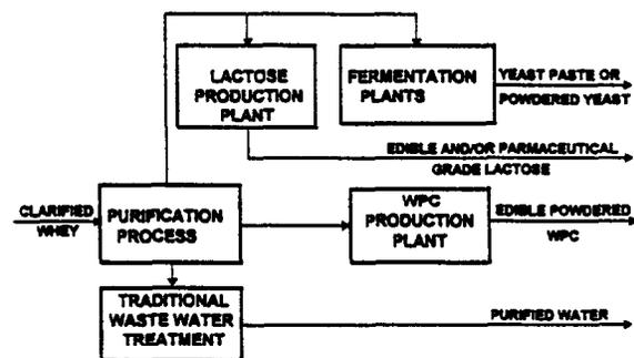
Fig. 1. Block diagram of a whey purification process integrated with other manufacturing processes at different levels.
