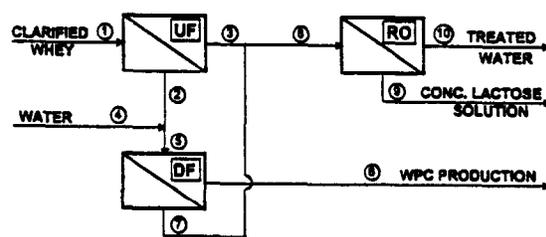
Fig. 2. Flow diagram of the whey treatment process.
