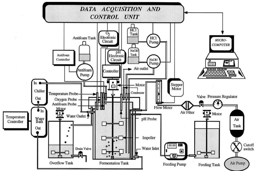
Fig. 2. Experimental apparatus.
