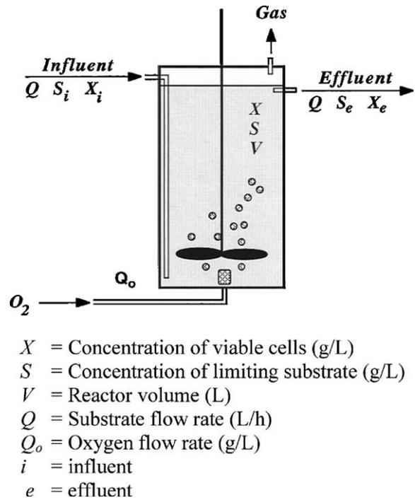
Fig. 1. Schematic of an aerobic continuous fermentation system.
