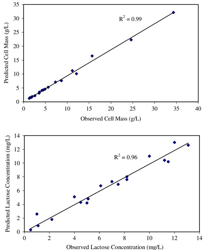
Fig. 7. Comparison of predicted and observed values of lactose concentration and cell mass.
