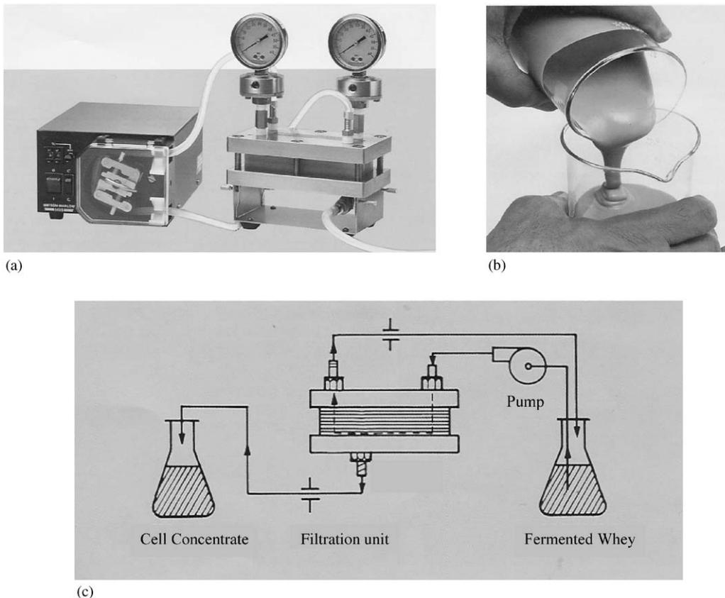
Fig. 2. Ultrafiltration system: (a) Model TM-100 filtration unit with Model 502S/R170 peristaltic pump; (b) concentrated yeast cell culture; (c) ultrafiltration unit in operation.
