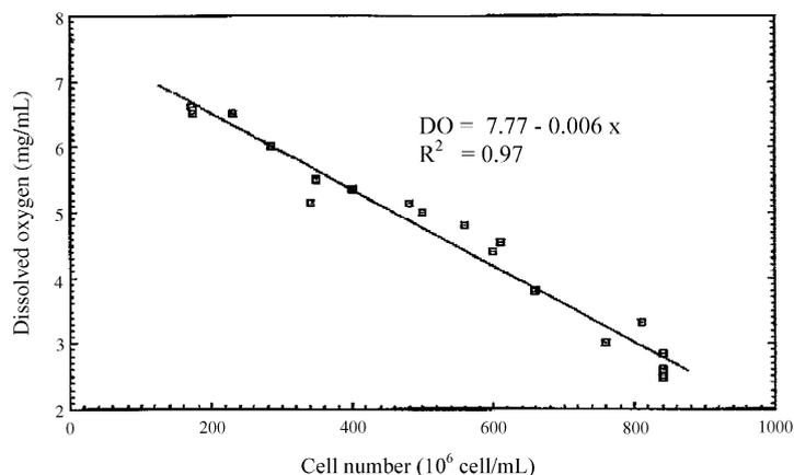
Fig. 4. Effect of cell number on dissolved oxygen.
