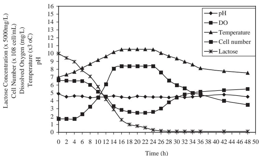
Fig. 3. The pH, temperature, dissolved oxygen concentration, cell number and lactose concentration measured during the batch culture operation.
