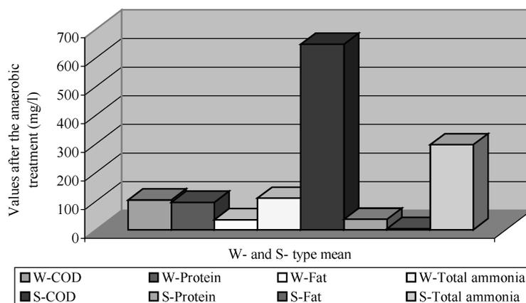
**Figure 4b** Final chemical characteristics of W- and S-type wastewaters after the anaerobic treatment (Adapted from Vidal et al., 2000).
