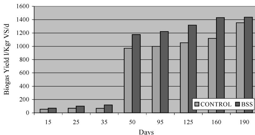
**Figure 2b** Comparison of start up performance between conventional and BSS-ST reactors regarding biogas production. (Adapted from Ramasamy, Abbasi, 2000)
