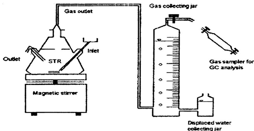
**Figure 1** A typical stirred tank reactor (STR) (Ramasamy and Abbasi, 2000).
