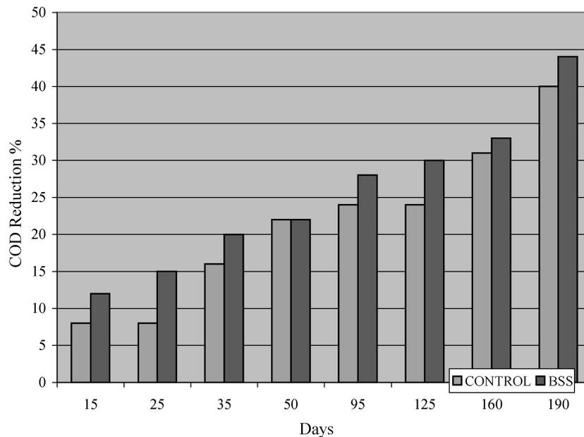
**Figure 2a** Comparison of start up performance between conventional and BSS-ST reactors regarding COD reduction (Adapted from Ramasamy and Abbasi, 2000).
