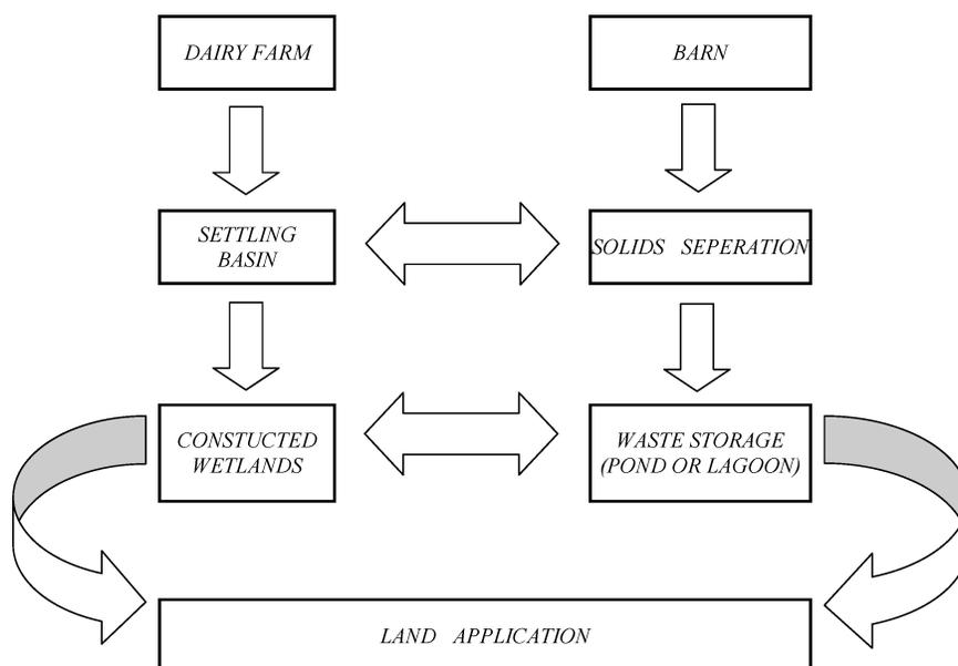
**Figure 5** Proposed scheme for the handling operations for the dairy farm wastewaters (adapted from Cronk, 1996, and NRCSB, 1992).
