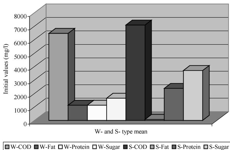
**Figure 4a** Initial chemical characteristics of W- and S-type wastewaters before the anaerobic treatment (Adapted from Vidal et al., 2000)
